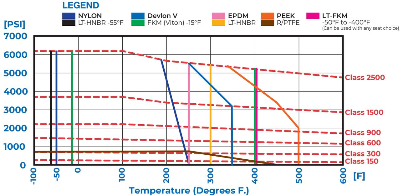
\*The Pressure/Temperature Limits of any valve are dependent upon the materials selected along with the seat/seal of choice.
