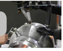
The largest hydro test stand gives us the capability of assembling and testing up through 42" valves.
