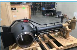
ISV's trunnion valves with high lead extensions. ISV can tailor the design to each end user's specification and provide the special coatings usually associated with buried service.
