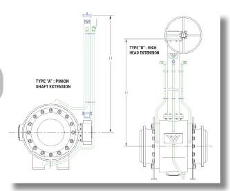
30" ANSI 150 ISV's trunnion with an actuator as specified by our customer.
